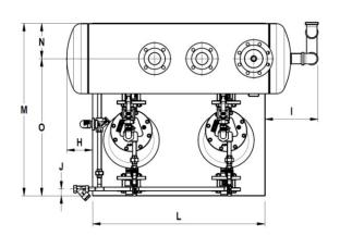
LIMITING CONDITIONS: Receiver - Max. operating pressure: 0,5 bar.
